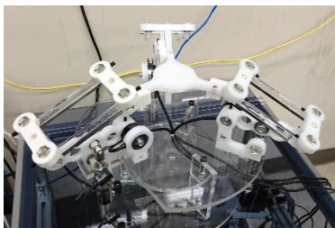
Fig.3 Force display device with pneumatic servo
